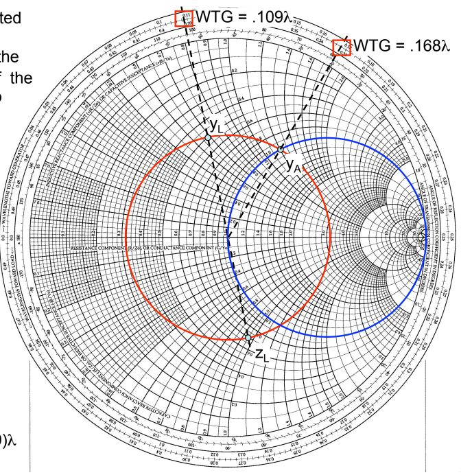
A 50- $\Omega$  T-L is terminated in an impedance of  $Z_L = 35 - j47.5$ . Find the position and length of the short-circuited stub to match it.
