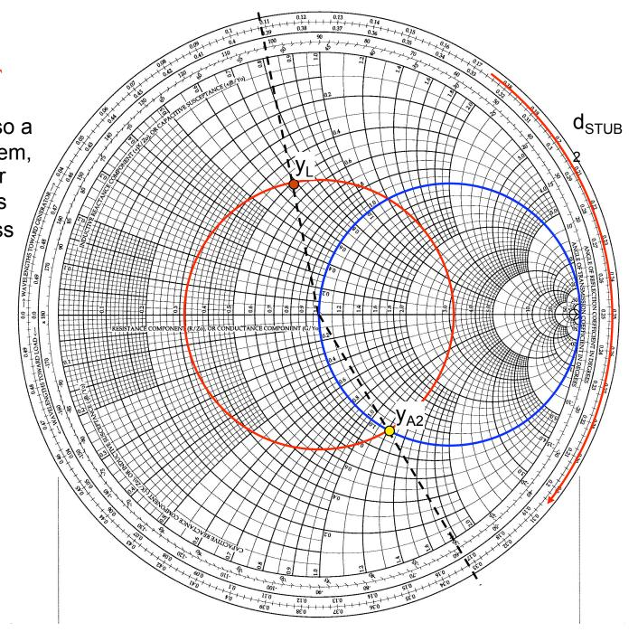
STUB.C ∠b<sub>A</sub> 1) Find  $y_L$ 2) Rotate towards generator until intersection with VAVELENCTHS TON g=1 circle ( $d_{STUB}$ ) 3) Read off b<sub>A</sub> 4) Find  $b_{STUB}$ 5) Rotate towards load until stub termination is reached ( $L_{STUB}$ ) STUB, SC ants **b**<sub>STUB</sub>
