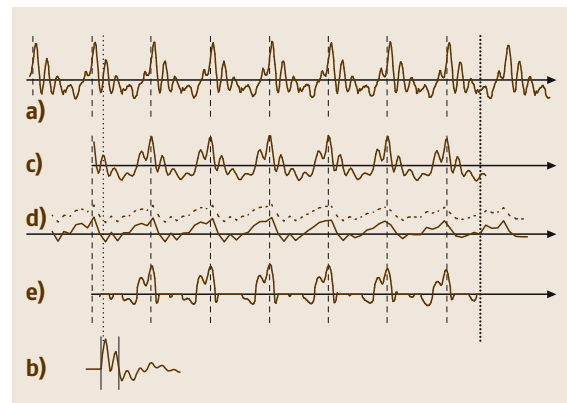
Fig. 10.11a–e Determining the instant of glottal closure via a maximum-likelihood criterion [10.91, 92]: example of performance. (a) Signal frame (45 ms); (b) impulse response h(n) of the vocal tract, estimated by linear prediction; (c) correlation function c(n) ; (d) envelope e(n) (dotted line) and high-pass filtered envelope; (e) product of c(n) and the filtered envelope
