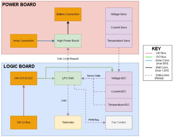
Figure 2: Block diagram of MPPTs
