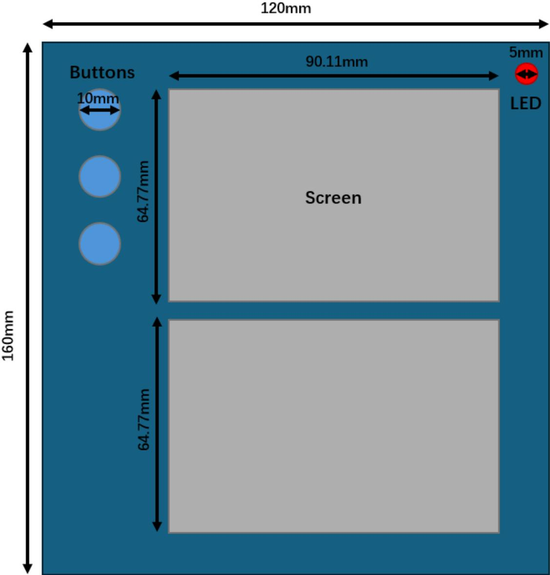
Figure 3: Physical dimensions of the *JargonJolt*
