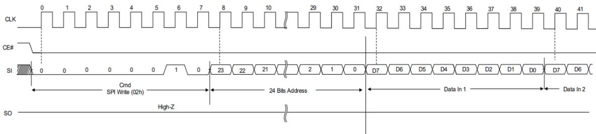
Figure 9: Timing diagram for writing to IS66WVS4M8ALL
