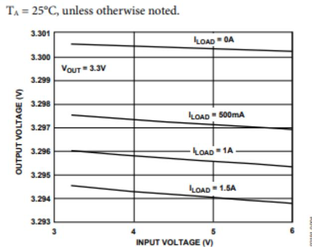
Figure 6: ADP3339 Voltage Input/Output curves with current load lines
