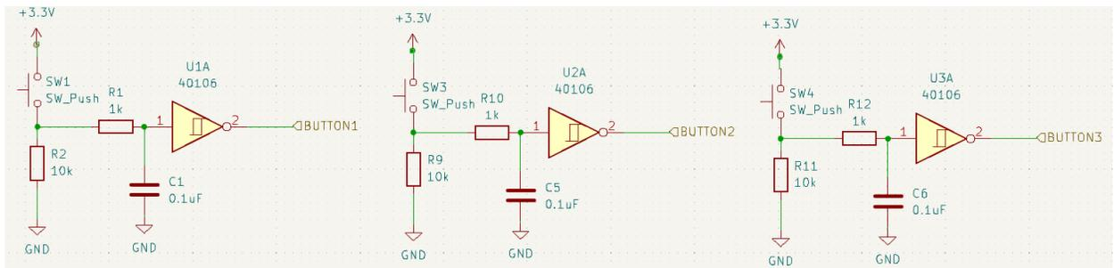
Figure 7: Schematic of face buttons
