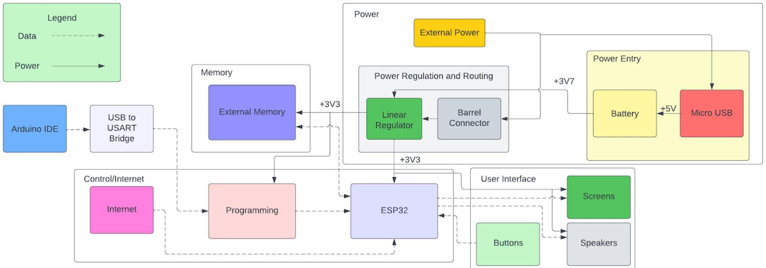
Figure 2: High level block diagram for *JargonJolt*
