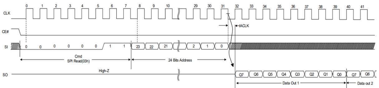
Figure 8: Timing diagram for reading from IS66WVS4M8ALL
