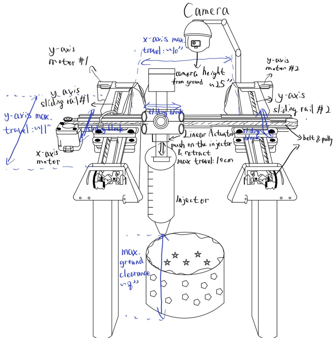
Fig. 4 Fully labeled physical diagram
