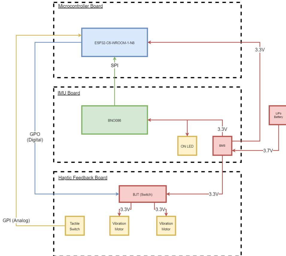
Figure 2: Block Diagram
